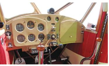
The neatly finished command center — note the chrome control sticks and Fairchild rudder pedals.
